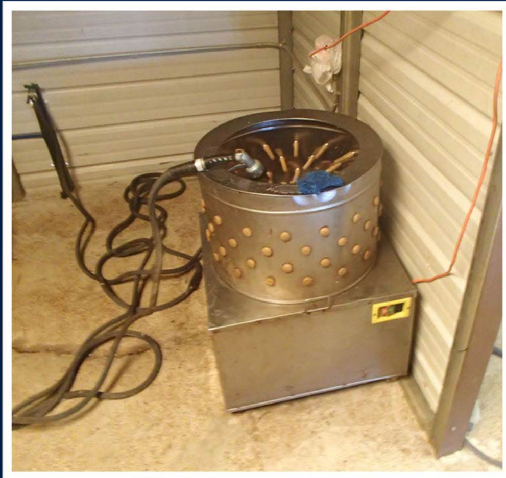
Actively processing chicken & goat meat shop with a chicken plucker and a goat scalding machine. Photos taken by Gary Balthrop.
