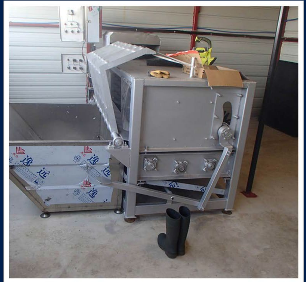
Actively processing chicken & goat meat shop with a chicken plucker and a goat scalding machine. Photos taken by Gary Balthrop.
